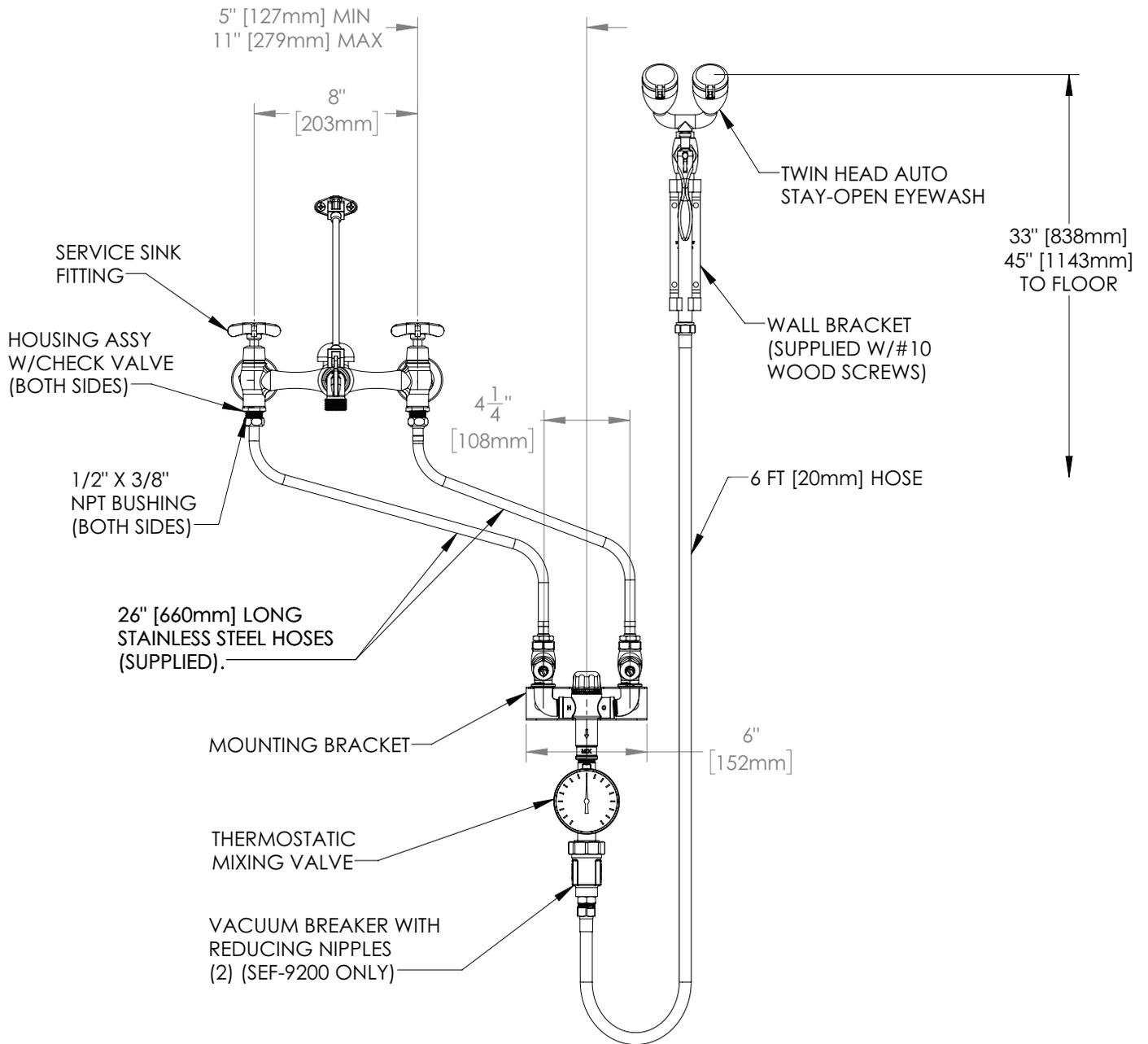
1. All dimensions are in inches (millimeters) unless otherwise specified and are subject to change without notice. 2. Mixing valve can be hard piped with unions.
